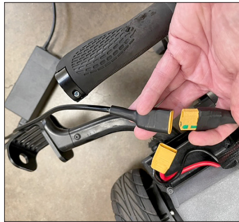
Figure P: Battery connected to charger.
