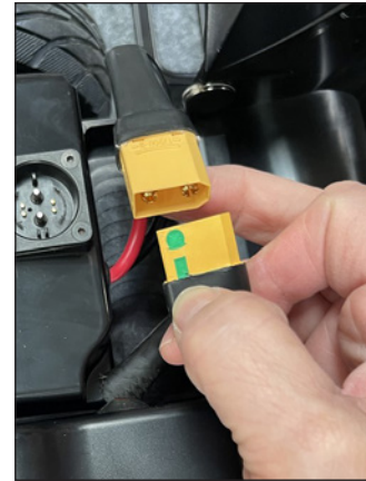
Figure N: Battery disconnected.
